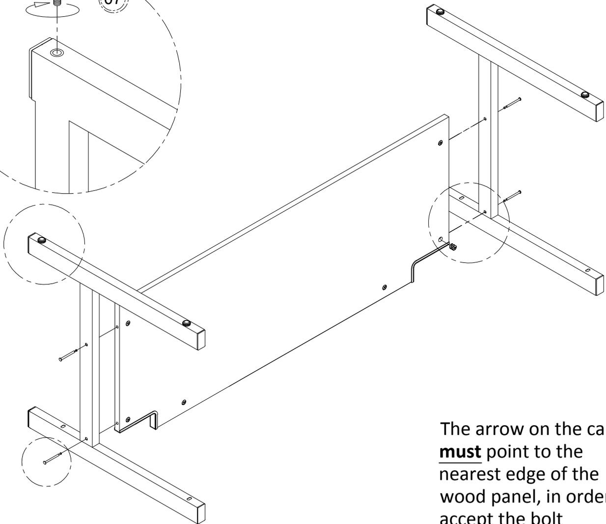
The arrow on the cam **must** point to the nearest edge of the wood panel, in order to accept the bolt
